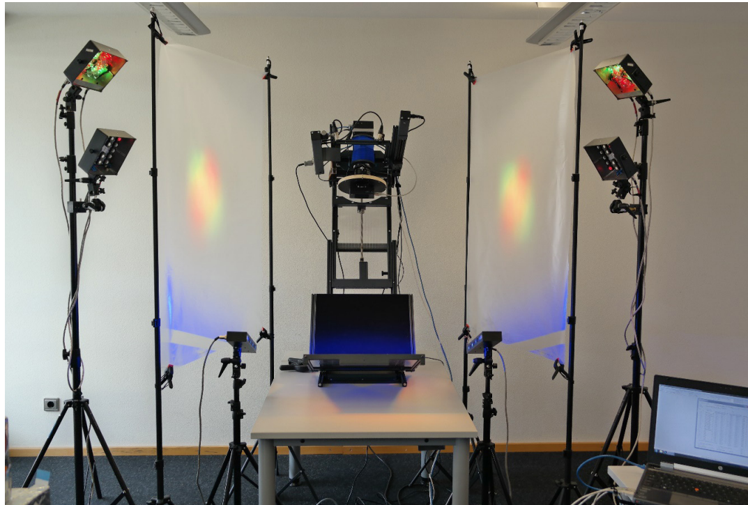
Fig. III.1: CSMC camera system with LED lighting
