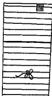
Uncut sheet: Horizontal chain lines; watermark near or below center of one-half of oblong
