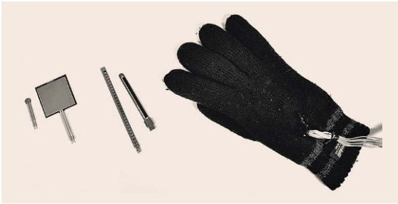
Fig. 38.9 Examples of small and large force and bend sensors ( left ) and a custom-built glove with similar sensors built in ( right )
