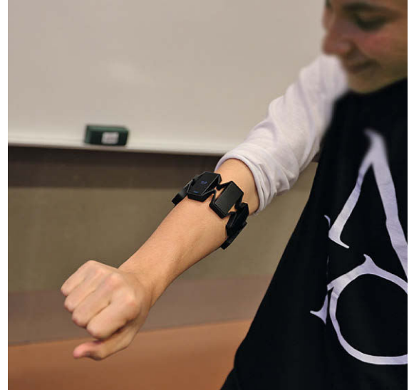
Fig. 38.13 An example of music interaction with the commercially available Myo armband, which contains eight EMG sensors, accelerometers and gyroscopes (Photo: Kristian Nymoen)
