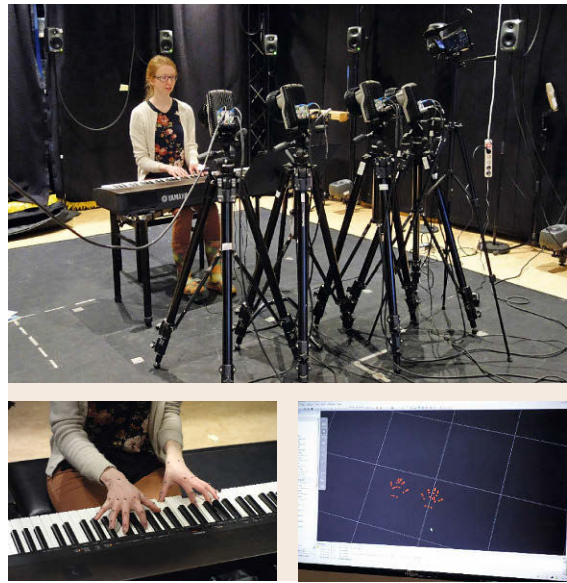
Fig. 38.8 Setup for motion capture of pianist Christina Kobb. In addition to the cameras placed in front, there are also cameras placed behind the pianist to capture the motion in three dimensions
