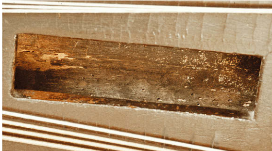
Fig. 4.9 Worm holes in the soundboard (probably Paulownia) of a Ming dynasty guqin, seen through the tonehole on the underside
