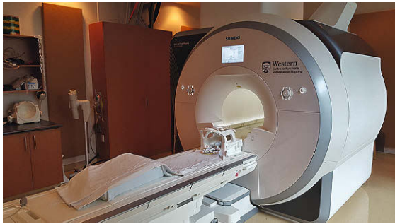
Fig. 27.6 A functional magnetic resonance imaging (fMRI) machine. Participants lie on the bed, which is moved until their head is in strong magnetic field in the bore, the small hole in the middle of the round structure. The coil (small round cage-like structure on the bed, close to the magnet) is used to detect changes in the blood-oxygen-level-dependent (BOLD) signal, which denotes brain activity (Photo: Siemens 3-Tesla Prisma MRI scanner with 64-channel head coil, housed at the Centre for Functional and Metabolic Mapping at The University of Western Ontario, London, Ontario, Canada)
